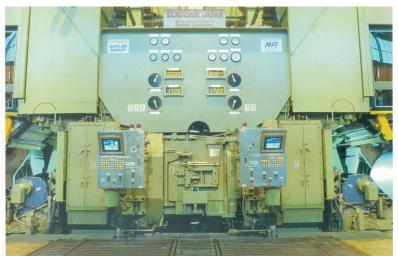
There are many other applications for which this extra heavy mill can be used, such as; stainless breakdown, production of wide, low carbon sheets, and rolling of extra wide material for the aircraft industry. The unique design of the Sendzimir mill allows building the ZR 21 mill section for rolling strip in widths of approximately 74".
