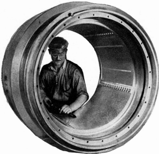
Figure 22 — Oil lubricated plain type roll neck bearing.
