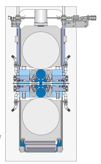
Essentially a 6-high mill with side-supported work rolls, the Z-high mill permits a greater variety and quality of product. Its retrofit design, allowing it to use an existing 4-high housing, minimizes the capital outlay.
