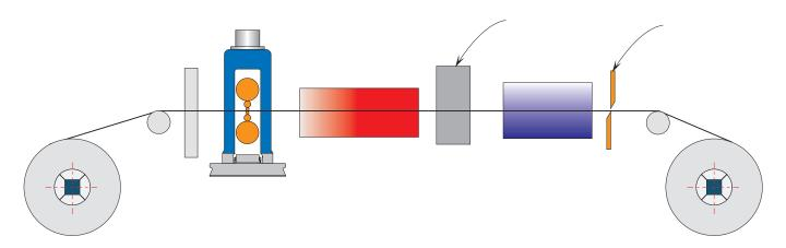
could be simultaneously changed with minimum risk of surface damage to rolls or strip. Furthermore, the strip can be stopped for an extra few seconds just after the weld passes through the roll bite, allowing time for the mill settings to be adjusted, if necessary. The mill and uncoiler would then be accelerated to refill the storage looper.
