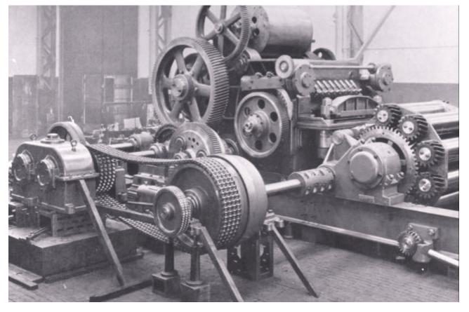
Figure 1. The first Sendzimir mill, built in 1932 in Poland
