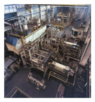
Figure 5. Two-stand Z-High mills in the DRAP line at J&L Specialty Metals, Midland, Pennsylvania, USA.
