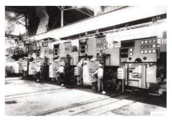
Figure 2. The first Sendzimir tandem mill, built in 1969 for Nisshin Steel
