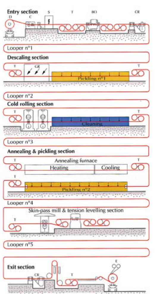
**Figure 4. Two Sendzimir Z-High mills are at the core of Ugine's new process line in Isbergues, France (picture courtesy of Metals Journal)**
