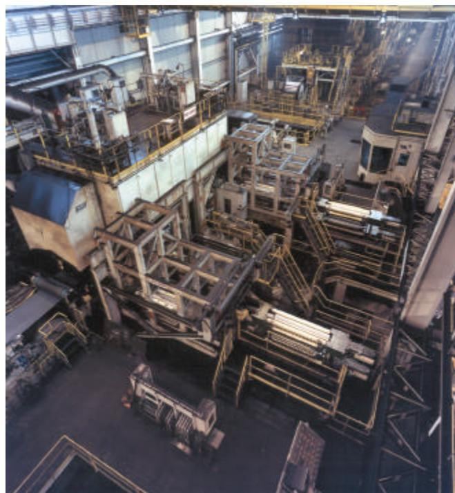
**Figure 5. Two-stand Z-High mills in the DRAP line at J&L Specialty Metals, Midland, Pennsylvania, USA.**
