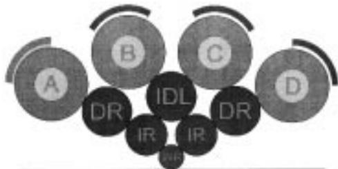
Fig. 3 — Sendzimir 20-h mill with eccentric rings on B and C shaft saddles to achieve dynamic crown control.
